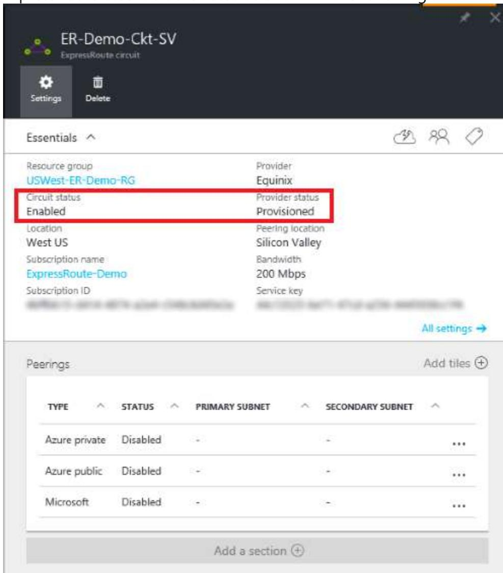
In the ExpressRoute Essentials, Circuit status indicates the status of the circuit on the Microsoft side. Provider status indicates if the circuit has been Provisioned/Not provisioned on the service-provider side.
