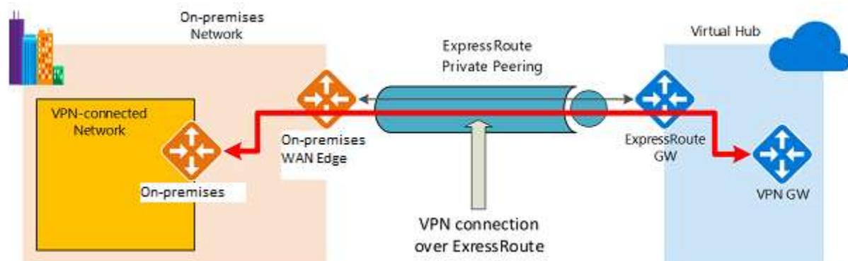
The diagram shows a network within the on-premises network connected to the Azure hub VPN gateway over ExpressRoute private peering. The connectivity establishment is straightforward:
